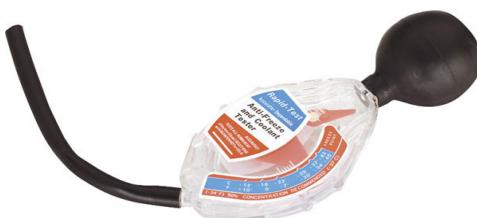
Checks condition of coolant antifreeze, hot or cold. Freeze protection level is indicated by the number of the six large coloured discs which float in the sample. Easy-to-read temperature table on the virtually unbreakable plastic body.
