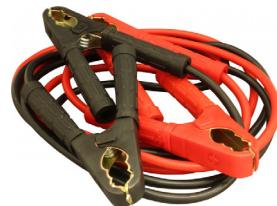
Professional automotive booster cable. 100% copper suitable for engine size up to maximum of 4000cc. CSA 16mm<sup>2</sup>. Peak output 400A. Starting output 250A. Oil, acid & heat resistant PVC. Length: 3 metres.
